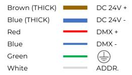
All wire terminations must be enclosed within a waterproof junction box to ensure safe and reliable connections.
