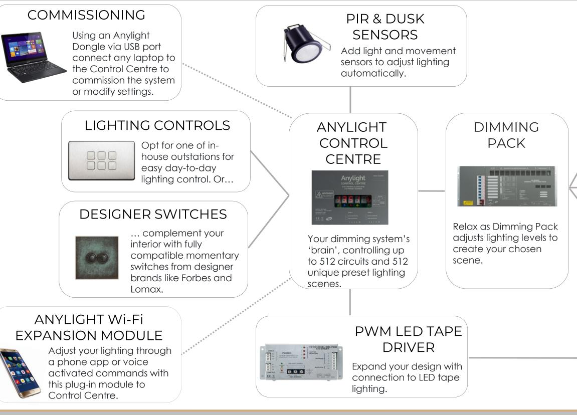
The above diagram represents possible set up for a dimming system with the range of products available from ZICO by Anytronics. Additional products may be required based on the individual set up.
